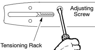
4. Slide guide bar on bar bolts until guide bar stops against clutch drum sprocket.
