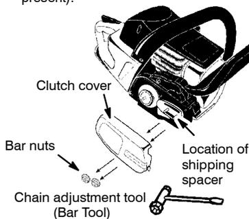
3. Turn adjusting screw on bar counterclockwise to move the tensioning rack as far as it will go toward the front of the bar.
